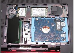
Pry the accessory plate up from the back of the laptop by applying force upwards where the screw was removed.
