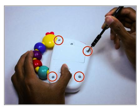
Using a screwdriver loosen the four screws connecting the body of the device together.
