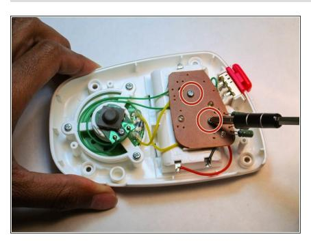
Using a screwdriver loosen the screws on the lights panel.
