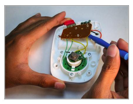
Using a plastic opening tool pop the light panel off. Be careful as to not rip any of the wires from the panel.
