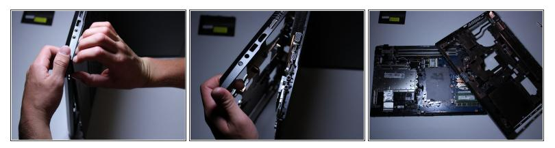
Gently pry around the edges with your fingers or a plastic separator to separate the middle layer from the base.
