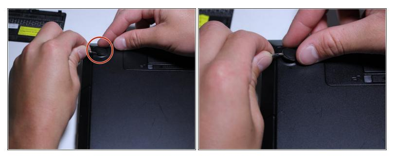
Pry off the rubber pads on the remaining three corners of the computer using the tip of the opening tool.
