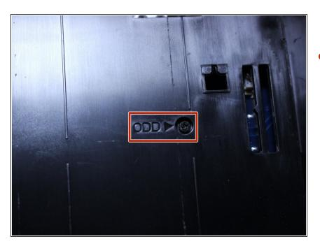
Using a Philips #00 screwdriver, remove the 6.5mm screw located next to the "ODD" print as indicated in the photo.
