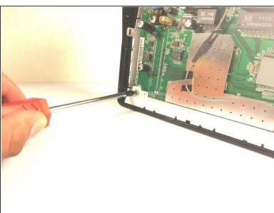
With your Phillips screwdriver, remove both screws by rotating in a counter-clockwise direction.
