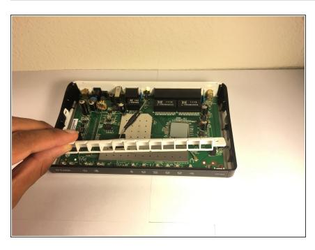
After removing the screws, lift the white LED cover up and off of the circuit board.
