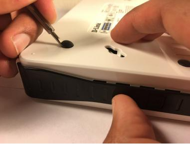
Using your flathead screwdriver or plastic opening tool, gently pry the top two screw covers out of the router's case.
