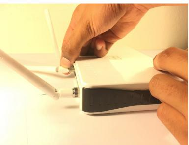
Start by removing the three antennas by twisting each one in a counter-clockwise direction when facing the back panel.
