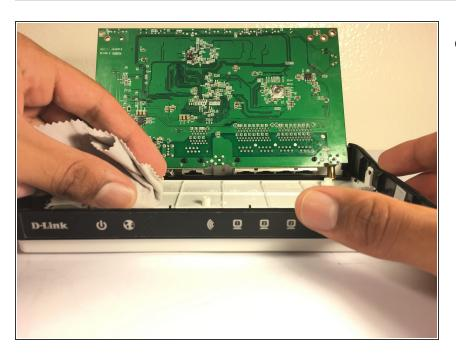
Wipe away any dust from the the vents to ensure proper airflow.
