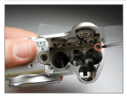
• Underneath the battery cover there is a 3.8 mm screw in the corner. Using the Phillips #00 screwdriver, remove this screw.
