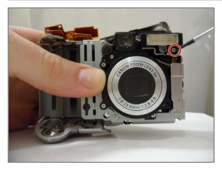
• Unscrew the 3.8 mm screw under the flash housing.
