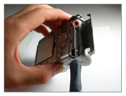
• Remove the Phillips #00 screw located inside the top of the memory card compartment.
