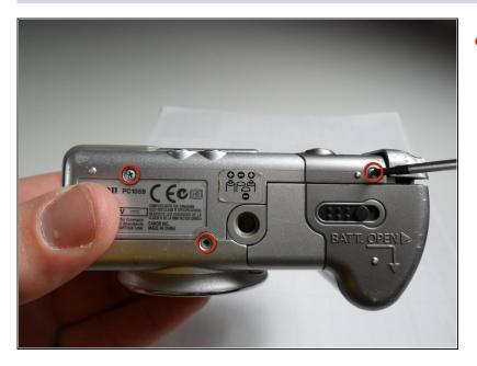
• Remove the three Phillips #00 screws from the bottom of the camera.
