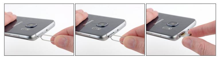
• Insert a paper clip or SIM eject tool into the hole in the SIM card slot on top of the phone.
