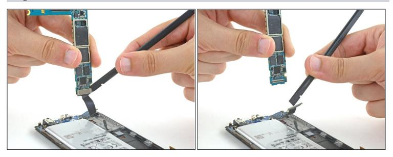
• Disconnect the daughterboard ribbon cable from the underside of the motherboard.
