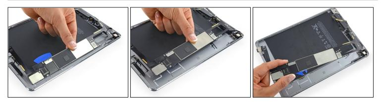
• Remove the logic board.
