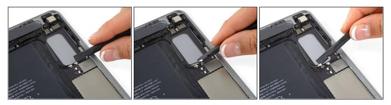
• Use a spudger to gently pry up the antenna cables from their sockets.
