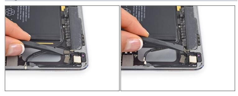
• Pry up the home button/microphone ribbon cable connector from its socket.
