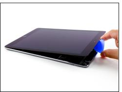
Twist the remaining pick by the front-facing camera to separate the top edge of the display assembly from the rear case.
