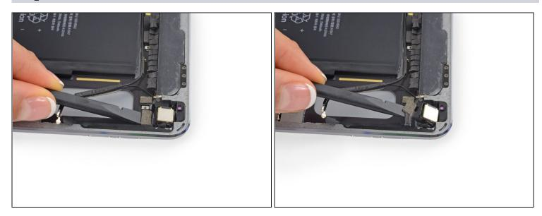
• Pry up the rear facing camera cable connector from its socket.
