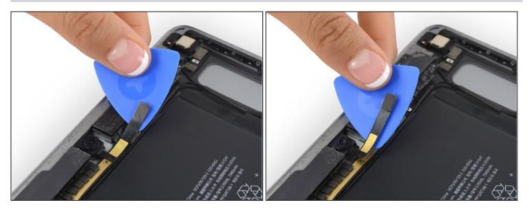
• Use an opening pick to break up the adhesive holding the FaceTime camera ribbon cable to the headphone jack cable underneath.
