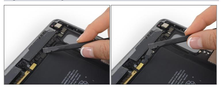
• Use the flat end of a spudger to disconnect the FaceTime camera cable from its socket on the logic board.
