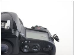
Using rubbing alcohol and a q-tip, clean the old adhesive strips and any residue off the LCD screen.
