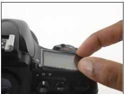
Press down on the edges of the display to ensure that the glass is strongly-adhered to the LCD.
