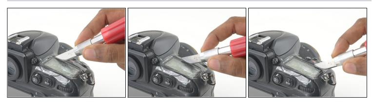
Slide the curved razor blade along the front edge of the LCD.
