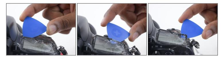
Slide the pick along the top edge of the glass, prying up on the glass against the plastic body as you go.
