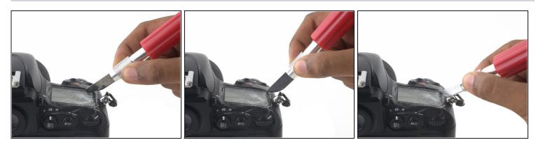
Bring the blade around the corner of the LCD closest to the shutter button.
