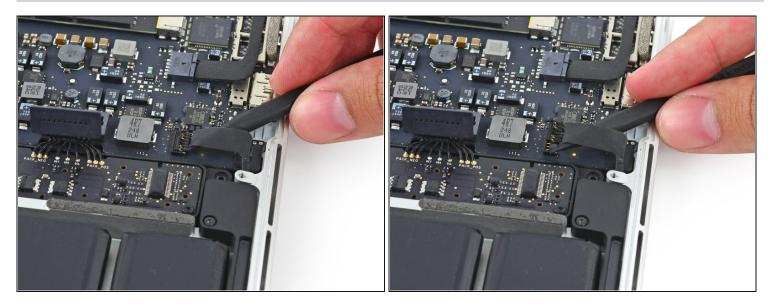
• Insert the tip of a spudger under the left speaker cable near the connector and lift it up out of its socket on the logic board.
