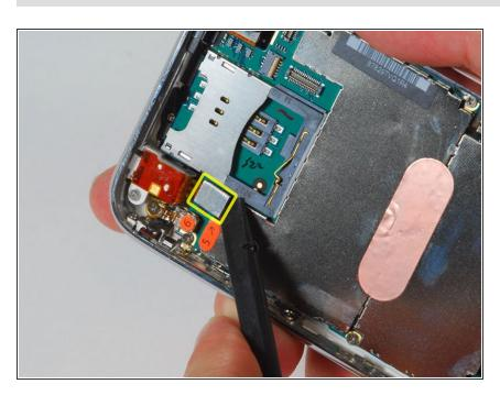
Use a spudger to disconnect the ribbon cable labeled "5."
