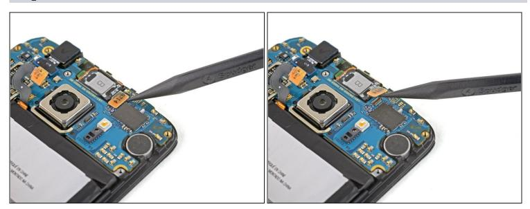
• Disconnect the earpiece speaker assembly cable connector from the motherboard.
