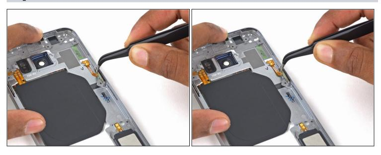
• Using the angled tweezers, grip the power button bracket and pull it out of its socket.
