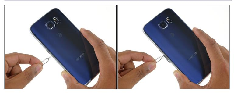
• Insert a paper clip or SIM eject tool into the hole in the SIM card slot on the power button side of the phone.
