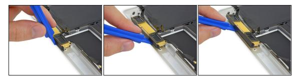
• Use a plastic opening tool to pry under the top edge of the right speaker, and separate it from the lower case.
