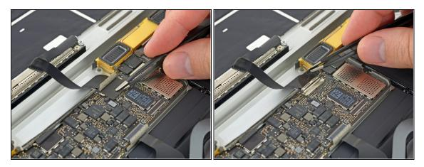
• Use tweezers to peel back the tape covering the display cable connector.
