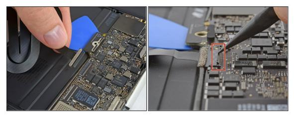
• Disconnect the trackpad cable from the logic board by gently pulling it straight out of its connector.
