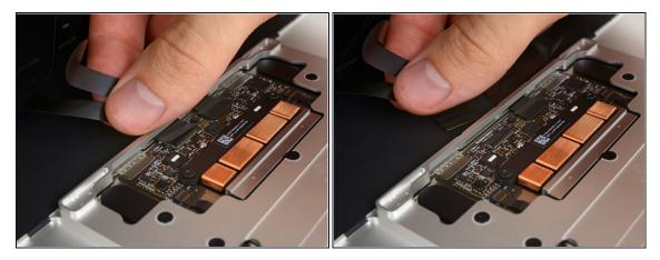
• Disconnect the trackpad ribbon cable from the trackpad by pulling it gently through its slot in the frame.
