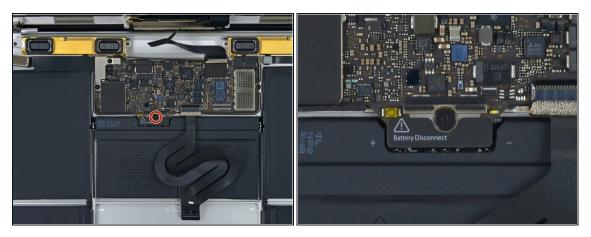
Remove the single 2.9 mm T5 Torx screw securing the battery connector to the logic board.
