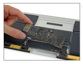
• Remove the logic board.
