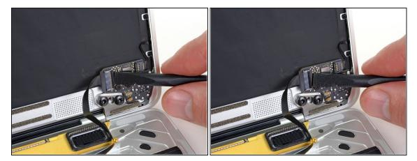
• Use a spudger to flip open the retaining flap on the audio jack board cable ZIF connector.
