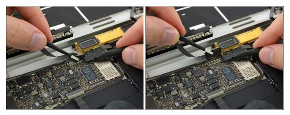
(i) It's possible the metal retaining flap on the display cable connector may flip open, remaining stuck to the tape.
