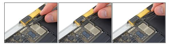
• Use tweezers to peel up the tape covering the two ZIF connectors—one for the right speaker cable, and one for the audio jack board cable.
