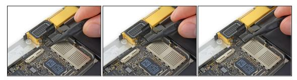
• Use the point of a spudger to flip up both ZIF connector retaining flaps.
