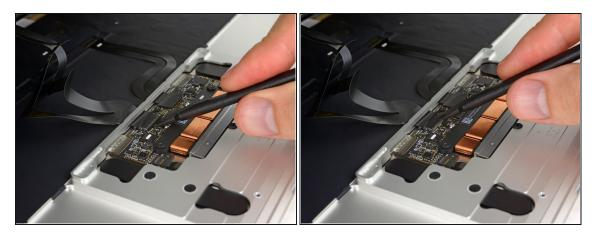
• Use a spudger to carefully flip up the retaining flap on the trackpad cable ZIF connector.
