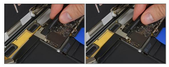
• Use the flat end of a spudger to disconnect the USB-C port cable bracket by prying it straight up from the logic board.
