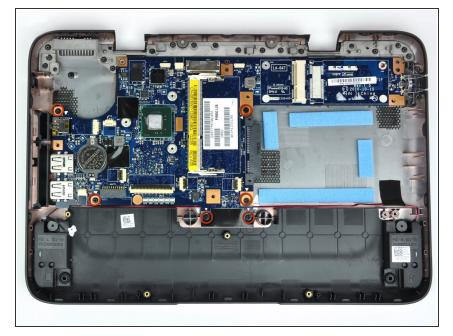
A handful of screws is all that remains between us and removing the motherboard from the lower case.
