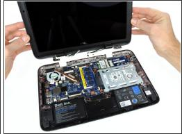
A few (6!) connectors and screws later, the display assembly comes free of the lower case.
