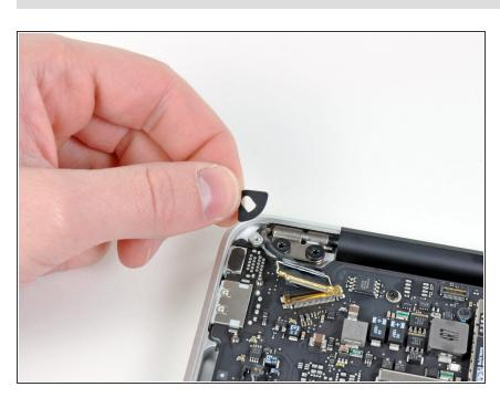
Remove the small rubber gasket from the corner of the upper case near the display data cable.
