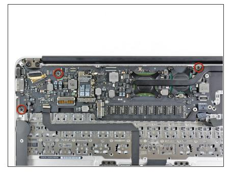
Remove the three 3.6 mm T5 Torx screws securing the logic board to the upper case.
