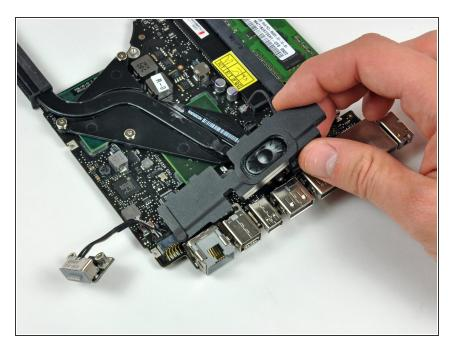
• Carefully peel the left speaker assembly off the adhesive securing it to the logic board.
