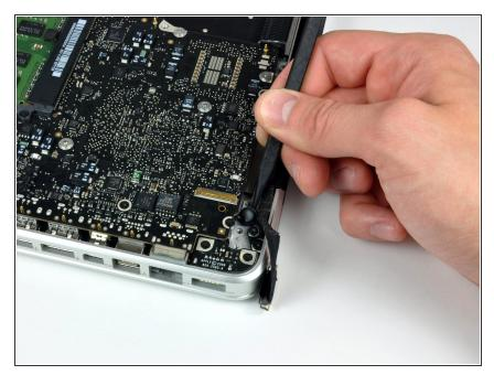
• Use the tip of a spudger to pry the microphone off the adhesive attaching it to the upper case.
