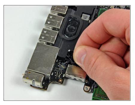
• Peel the tape off covering the microphone cable connector.
