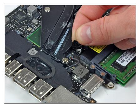
• Remove the strip of tape covering the left speaker cable connector.
