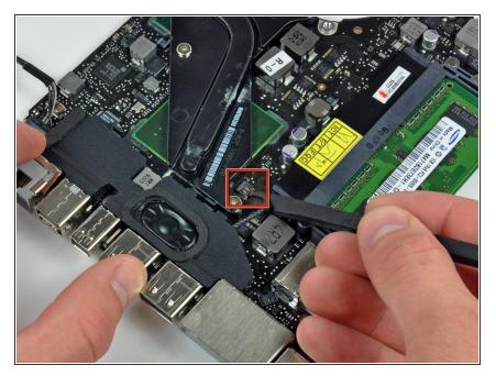
Use the flat end of a spudger to pry the left speaker connector up off the logic board.
