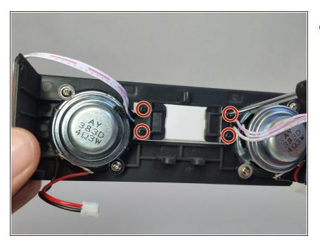
Remove four Phillips #0 head screws from the front panel.
