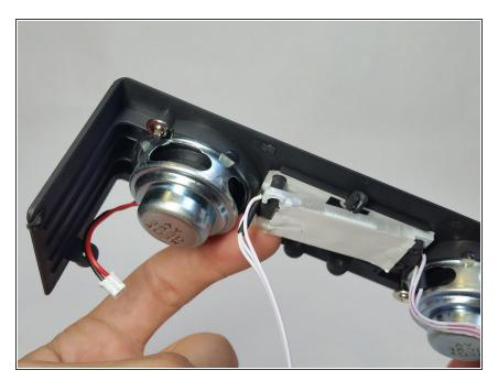
• Using the tip of your finger, gently separate the front panel display from its mount.
