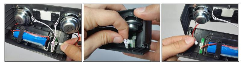
• Remove all cable connectors from the speaker motherboard.
