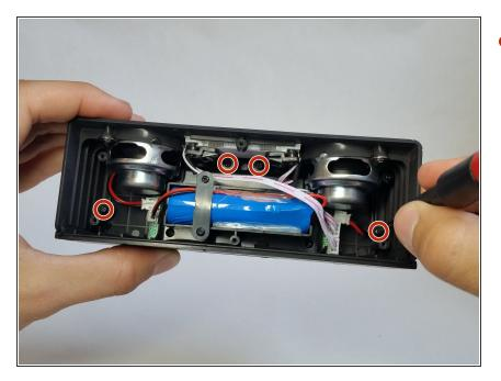
Remove four 9mm Phillips #0 head screws from the inside of the speaker case.
