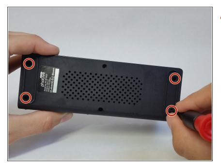
Remove four 9mm Phillips #0 head screws from the bottom of the speaker.
