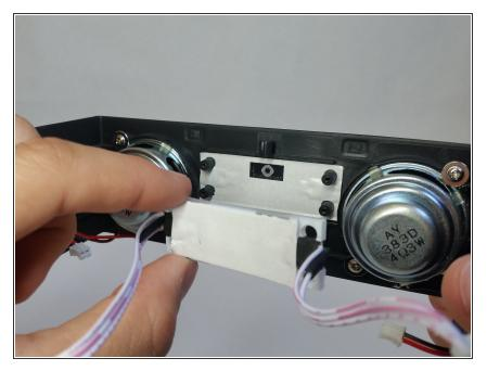
• Remove the front panel display.
