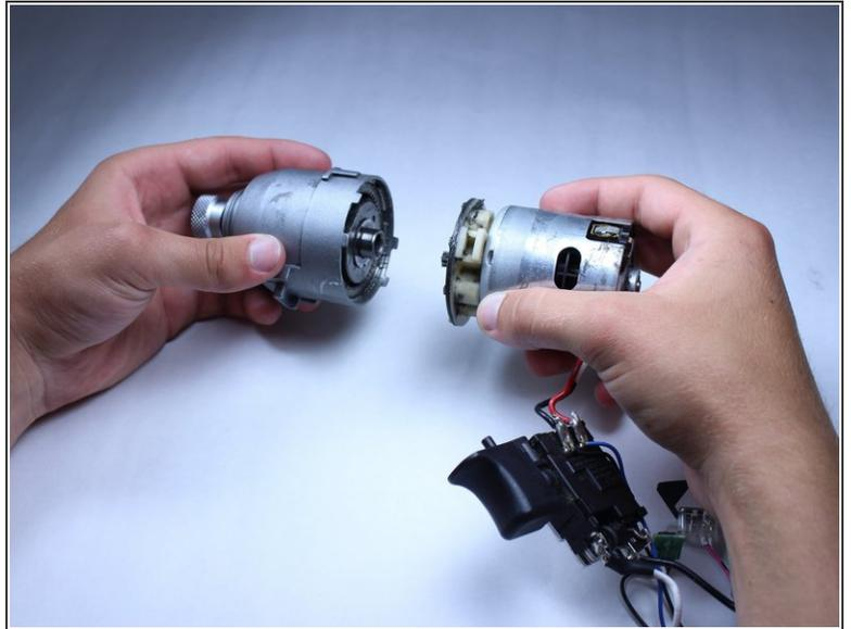
**!** Do not invert gear assembly! Keep gear assembly oriented so that the chuck is lower and the place the motor was attached is higher or else gears could fall out.
