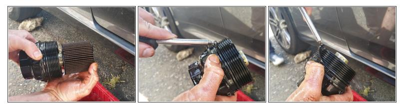
• Remove the paper filter from the filter cartridge; this is disposable. Use the flathead screwdriver to pry the o-ring off the cartridge.
