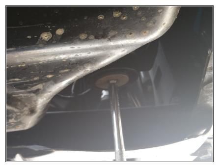
• Using the 3/8 inch socket wrench with extension, loosen the oil filter by putting the extension in the square hole in the filter and turning counterclockwise.
