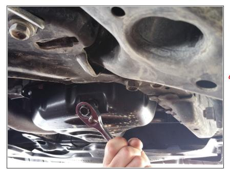
Allow oil to drain freely until drops of oil are slowly coming from the drain. Then re-tighten the oil drain plug using the 14mm socket wrench.
