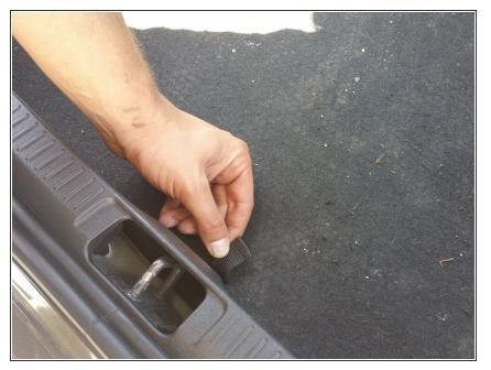
• Open the spare tire compartment in the trunk of the vehicle by pulling up on the black tab.
