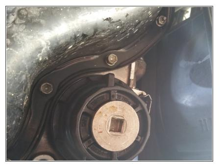
• Locate the oil filter. This is most accessible on your back from the front of the car. The filter should be about a foot closer to the front of the car from the oil drain plug.
