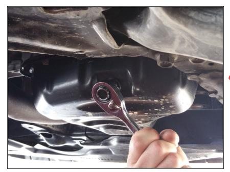
Using the 14mm socket wrench, loosen the drain plug by turning counterclockwise until you can turn the plug by hand.
