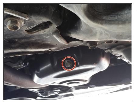
Once the jack stand is securely in place locate the engine oil drain plug. This is most accessible by crawling on your back from the front of the car.
