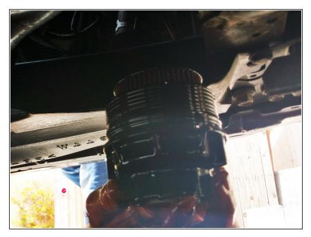
• Place the oil drain pan directly under the filter. Fully loosen the filter by hand until you are able to remove it from the vehicle.
