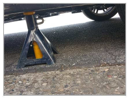
Lower the car onto the jack stand by turning the handle counterclockwise.
