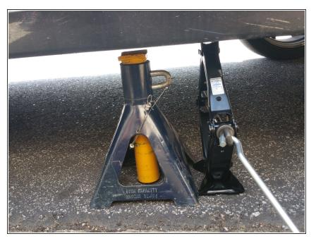
• Raise the car until the jack stand can fit underneath the frame. Place the jack stand under the frame as close to the jack as possible.
