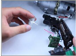
Cut the pink and white wires attached to the LED at a point that is a little more than 1/4 inch from the LED.
