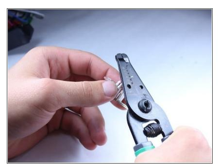
Strip the wires back about 1/4 inch on the LED.
