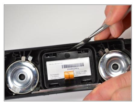
Once the motherboard has been removed, insert a standard metal spudger in between the outer and inner casing of the battery housing.
