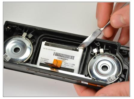
• There is a sticky adhesive on the bottom of the battery that keeps it in place. Insert a metal spudger under the side of the battery and gently begin to pry the battery away from the base.
