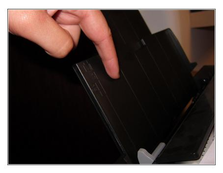
Pull down the parts that hold the paper on place. It's the best way to locate the roller and it's also more comfortable
