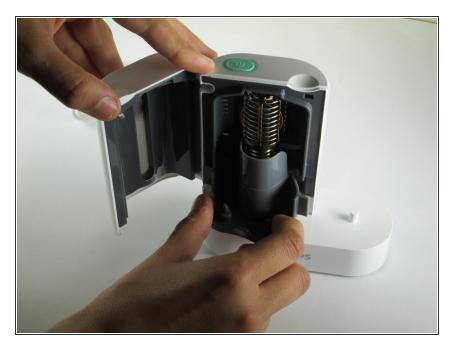
• Grip the sides of the plastic cover that is shielding the circuitry. Pull the cover outward to remove it from the sanitizer.
