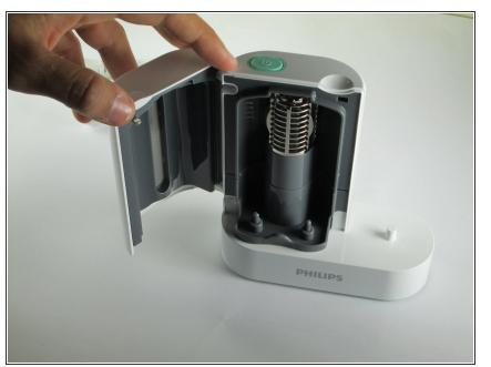
Before initiating the process, ensure that the sanitizer is not plugged into an outlet. Swing the door open to expose the interior of the sanitizing device.
