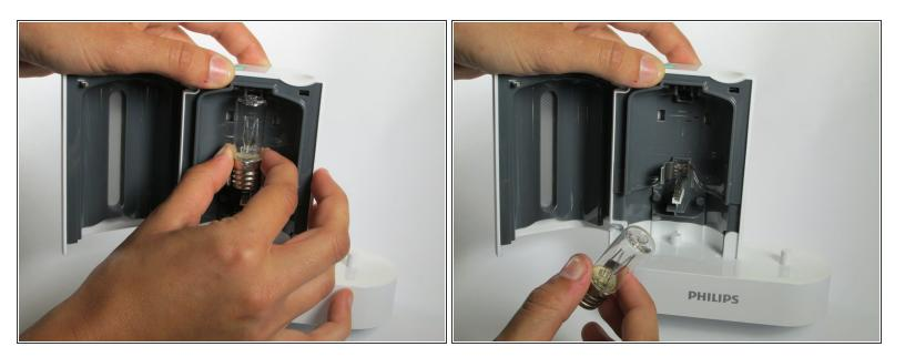
Before holding the light bulb, ensure that it is not warm due to previous use. Once that is confirmed, take a hold of the light bulb by the threaded surface and rotate it while pulling it outward. Have a compatible UV bulb to replace the old one.
