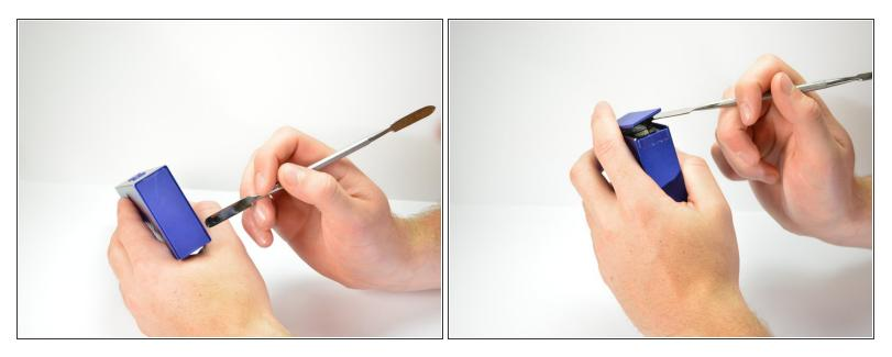
• Using the standard metal spudger, begin by prying at the bottom of the plain rubber end cap (the end without the USB or auxiliary input).
