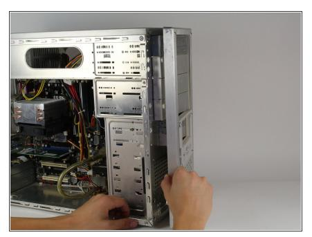
Disconnect the front panel from the computer face.
