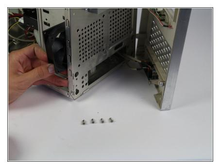
Slide the fan out from the side of the casing.
