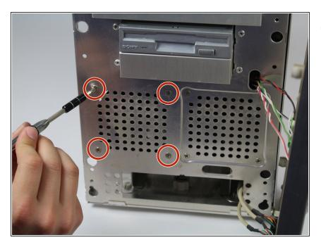
Remove four Phillips #2 head, 5mm screws holding in the fan.
