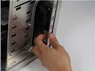
Push to unlatch three grey connectors on the front panel.
