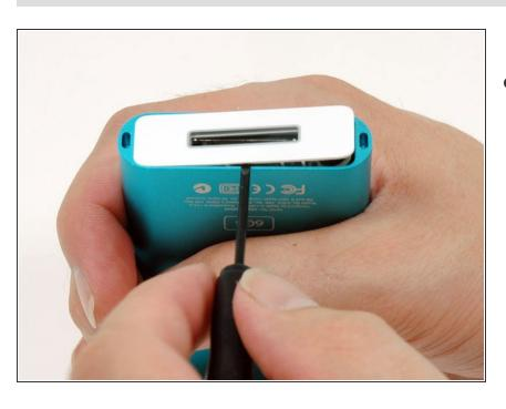
Carefully insert a small flathead screwdriver or <u>Jimmy</u> in the seam between the metal casing and white plastic bottom Use the screwdriver to pry up the white plastic bottom bezel. Be careful not to damage the soft plastic with your screwdriver.
