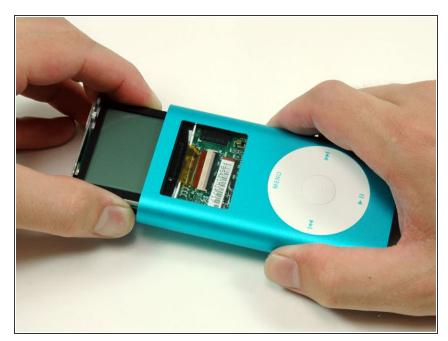
After pushing the logic board out sufficiently, gently grasp the logic board on either side of the display, and continue to slide the iPod out of its casing.
