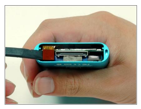
Use a spudger or the tip of your finger to carefully disconnect the orange click wheel ribbon from the logic board.
