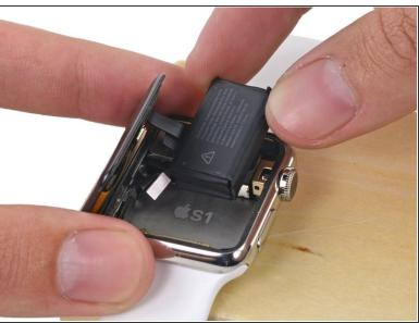
Rotate the battery counterclockwise to expose its connector.
