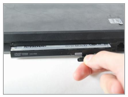
Grab onto the tab and pull away from the body of the ThinkPad. The tab should move out as far as seen in the picture.
