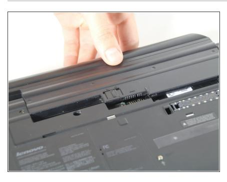
With the tab in the "unlock" position, gently slide the battery away from the body of the ThinkPad.
