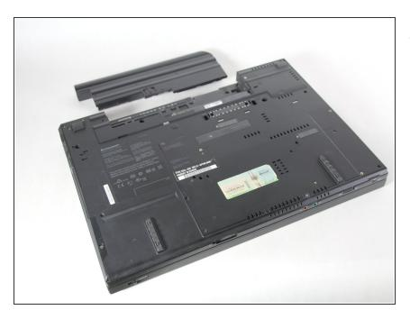
The battery is out! You can now replace it with the correct replacement battery and be on your way!
