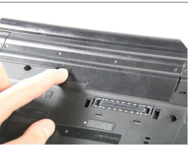
Slide the battery locking tab on the underside of the ThinkPad T500 to the right.
