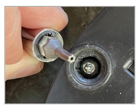
Also the front two screws are safety screws: they have a 6 sided star shape with a raised dimple in the center to prevent homebodies from casually opening the machine. (probably from the Sunbeam's (owns Mr. Coffee) legal dept.) Anyway you will need a security bit to remove the screws and not a phillips screw driver.
