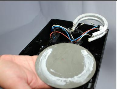
Push the heating plate up from below and remove.
