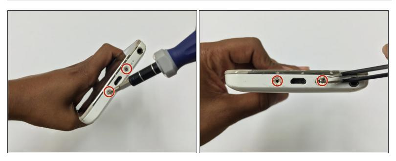
Using a Phillips head screwdriver, unscrew the two 10 mm screws located on either side of the charging port.
