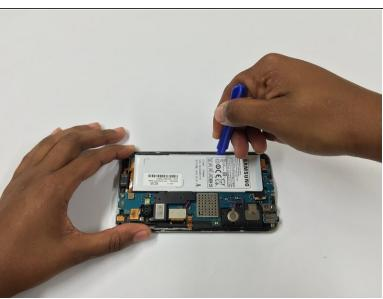
Using the plastic opening tool, apply an upward force to detach the battery and the tab attached to it.
