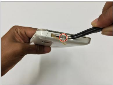
Remove the SD Memory Card before working on the device.
