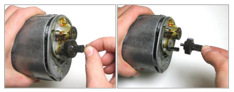
• Remove gear from the divider and add the new gear.
