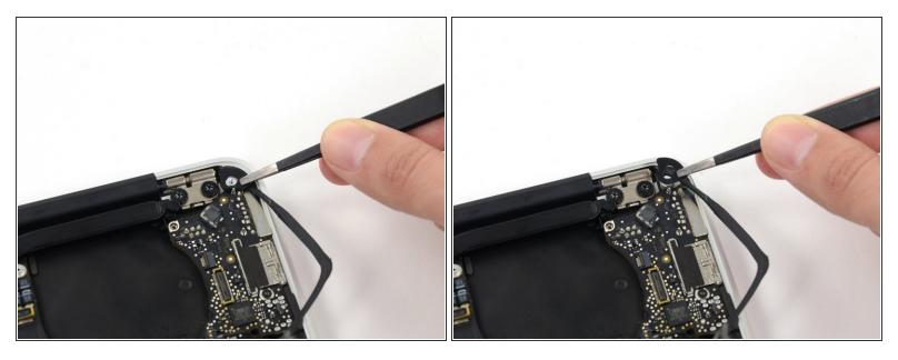
• Remove the small rubber gasket from the corner of the upper case nearest the I/O board.
