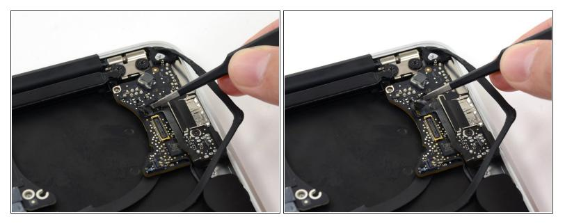
(i) If necessary, use tweezers to remove any tape covering the microphone cable ZIF connector.
