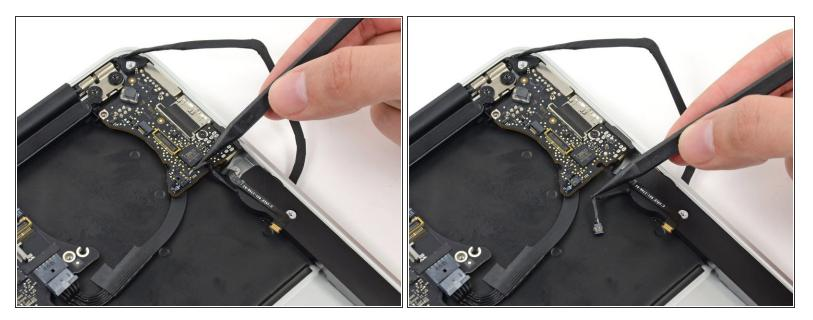
De-route the cable from its notch in the I/O board.
