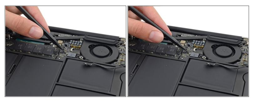
• Use the tip of a spudger to carefully flip up the retaining flap on the fan cable ZIF socket.
