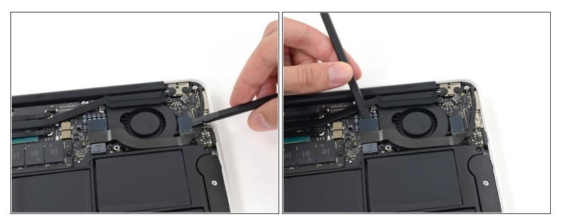
Use the flat end of a spudger to pry the left and right I/O board cable connectors up off their respective sockets on the I/O board.
