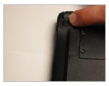
Unlock the battery by sliding the switch located near the left hinge to the left "unlocked" position.
