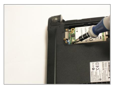
Remove the single 3.9 mm Phillips #1 screw from the bottom left of the wireless card.
