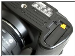
Insert the battery into the battery compartment at the bottom of the camera.
