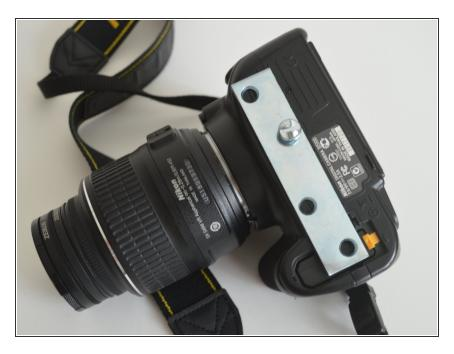
The metal bar should be attached and tightly secured.
