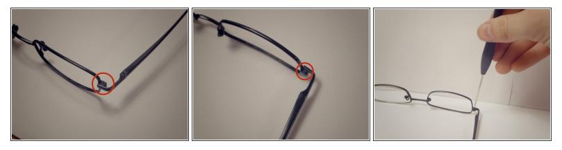
Locate the screw on the corner hinge of the glasses between the lens and the arms and unscrew it using the 1.5mm screwdriver by rotating counterclockwise.
