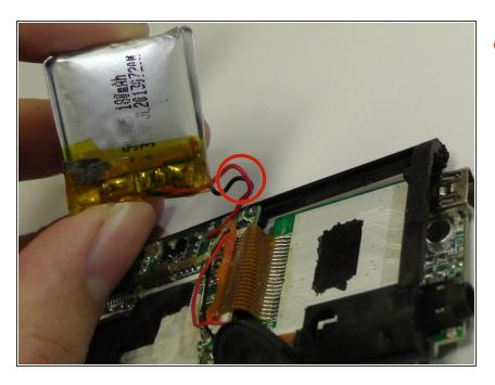
• Snip the wires using a wirecutter. Be careful not to nick the battery.
