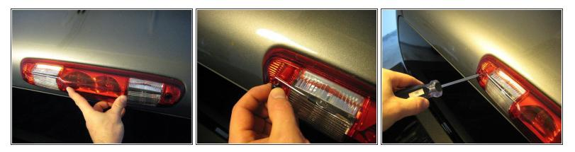
• Put back the light housing and screw in the two Philips screws.
