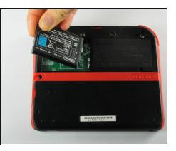
• Remove the battery from its housing by lifting it up from the side closest to the outside edge.
