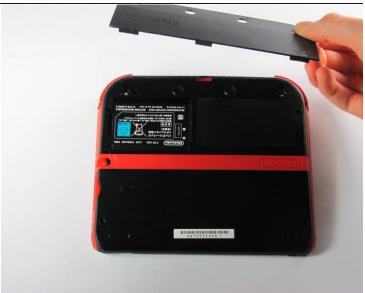
• Hinge the upper rear panel upwards and outwards to remove it.
