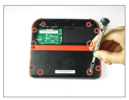
Remove the ten Phillips screws attaching the rear panel.
