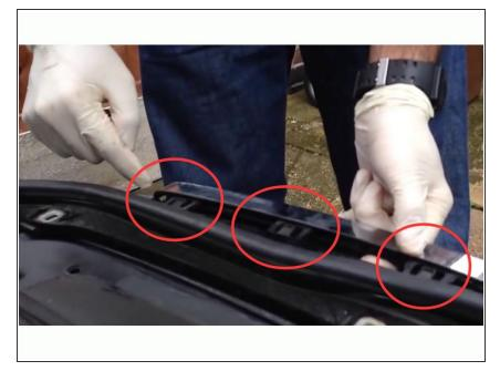
Detach the stock kidney grille from the clips holding it onto the BMW front bumper.
