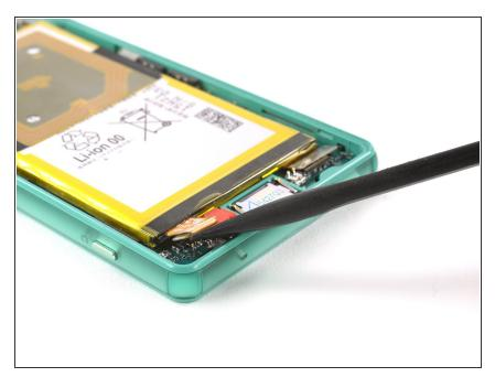
Disconnect the battery flex cable.
