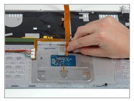
• Slide the orange keyboard backlight ribbon out of its connector.
