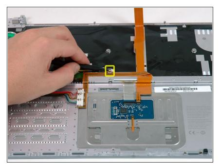
• Use a spudger or your finger to slide the keyboard backlight ribbon out of its connector.
