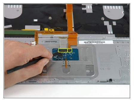
Use the tip of a spudger to flip up the black plastic flaps locking down the keyboard and keyboard backlight ribbon cables.
