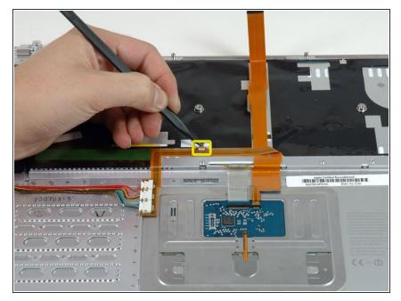
• Use the tip of a spudger to flip up the brown plastic flap locking down the keyboard backlight ribbon cable.
