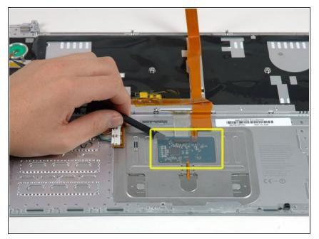
• Use a spudger to pry up the translucent plastic sheath covering the keyboard connector.
