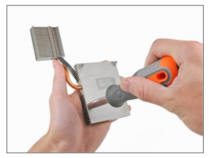
Use the 1/4" socket drive end of the included screwdriver with no bit inserted to remove the four X-clamp posts from both the CPU and GPU heatsinks.
