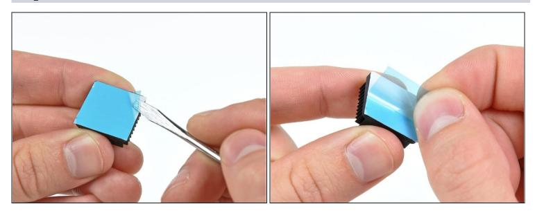
• Use the edge of your small flathead screwdriver or another thin and sharp object to carefully pull up a corner of the blue or white plastic sheet covering the adhesive on the bottom of both heat sinks.
