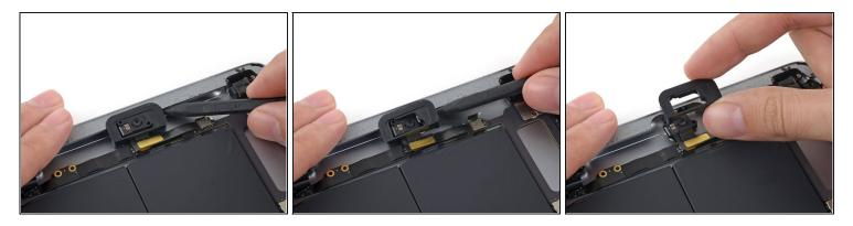
• Use the tip of a spudger to pry the front-facing camera housing up and lift it out of the case.
