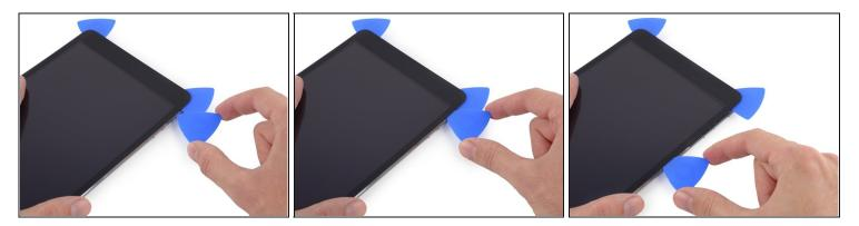
• Insert a new opening pick and slide it to the middle of the right edge of the iPad, releasing the adhesive as you go.
