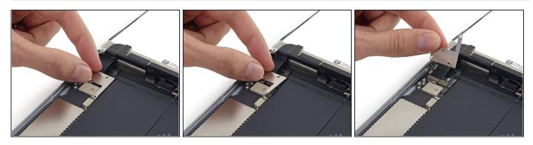
• Remove the display cable bracket from the iPad.
