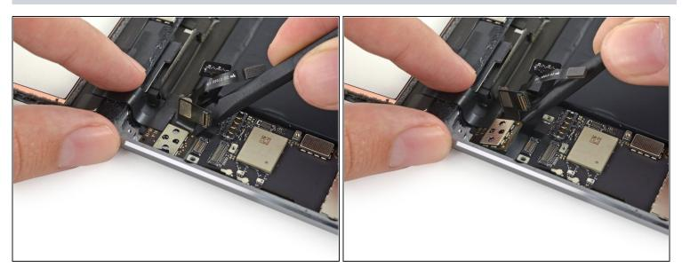
• Slide the flat end of a spudger under the battery side of the digitizer board to begin separating it from the rear case.
