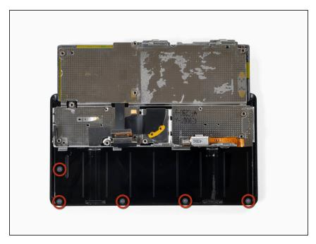
Remove the five 2.5 mm T3 Torx screws along the outer edge of the slider panel.
