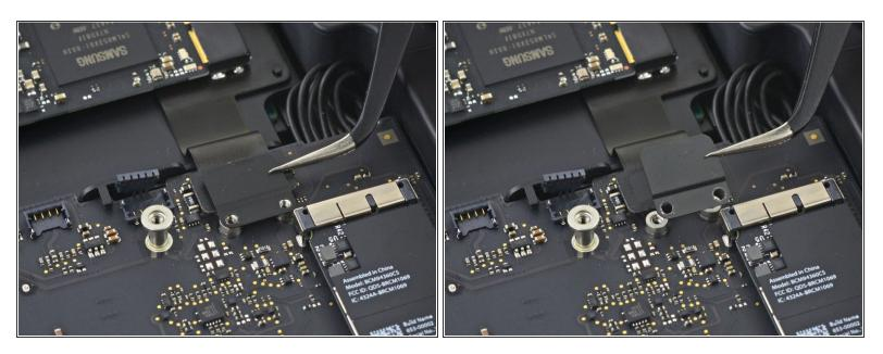
• Remove the PCIe SSD cable bracket.
