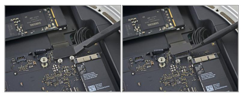
• Lift the PCIe SSD connector up off its socket.
