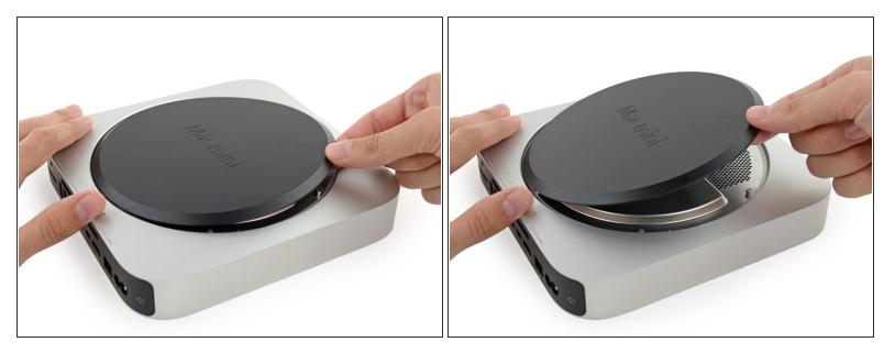
• Lift and remove the bottom cover.
