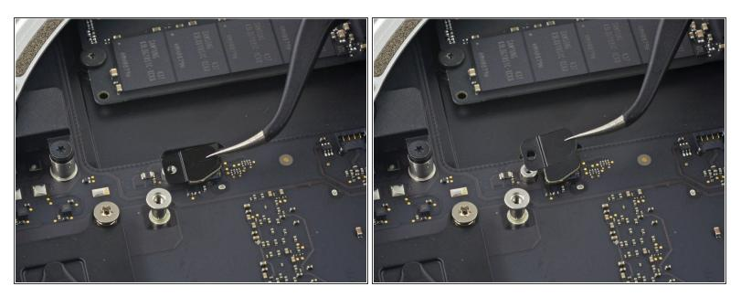
• Remove the SATA cable connector bracket.
