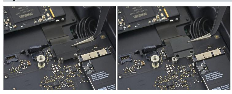
• Remove the PCIe SSD cable bracket.
