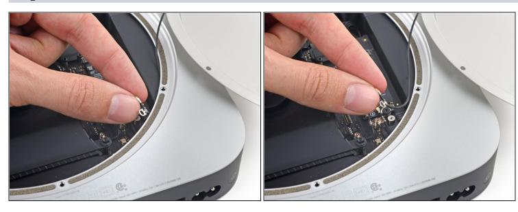
• Carefully pull the antenna cable out from the gap between the power supply and case.
