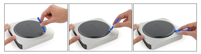
• Use the plastic opening tool to pry the bottom cover up off of the Mac mini.
