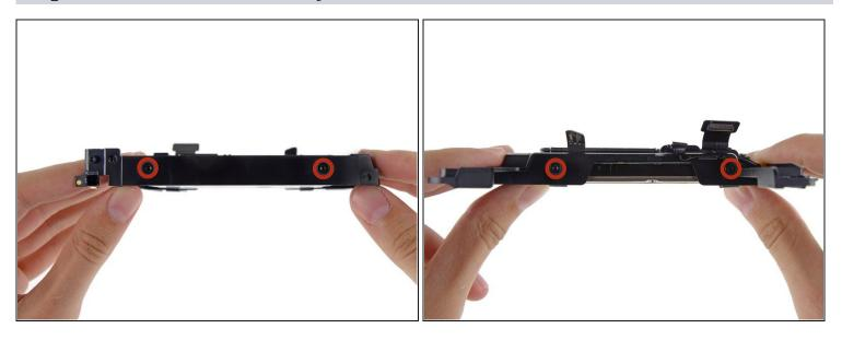
• Remove the four (two on each side) 6.5 mm T8 screws securing the hard drive to the drive tray.
