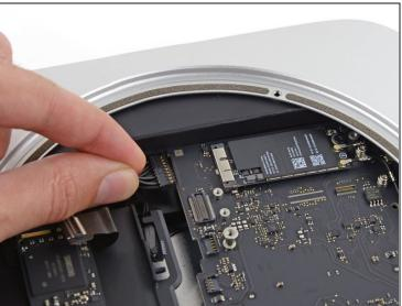
• Pull the DC-In cable connector straight out of its socket on the logic board.
