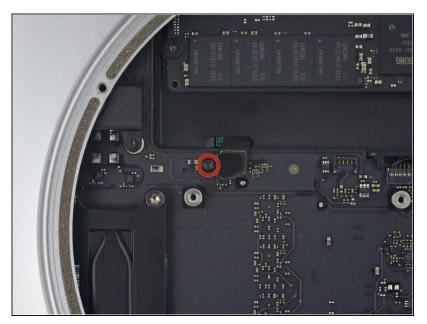
Remove the 2.6 mm T6 screw securing the SATA cable connector bracket.
