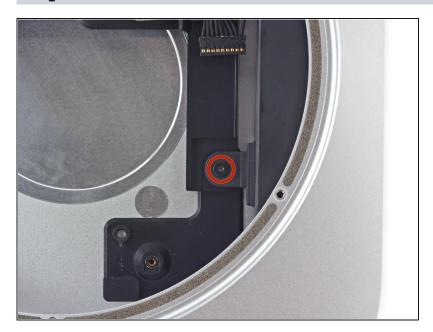
• Remove the 8 mm T6 screw securing the power supply.
