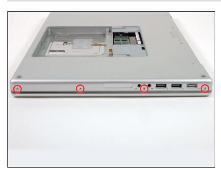
Rotate the computer 90 degrees again and remove the four Phillips screws from the side of the computer.
