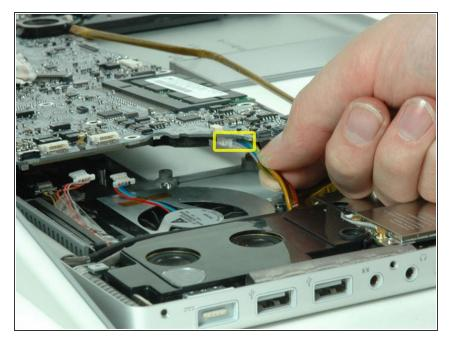
Lift up the left side of the logic board and disconnect the multi-colored power connector from the bottom of the board.
